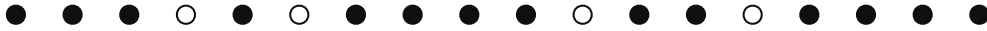
Figure 5.1: Partitioning N bosons into J possible states ( N = 14 and J = 5 shown). The N black dots represent bosons, while the J - 1 white dots represent markers separating the different single particle populations. Here n_1 = 3 , n_2 = 1 , n_3 = 4 , n_4 = 2 , and n_5 = 4 .
