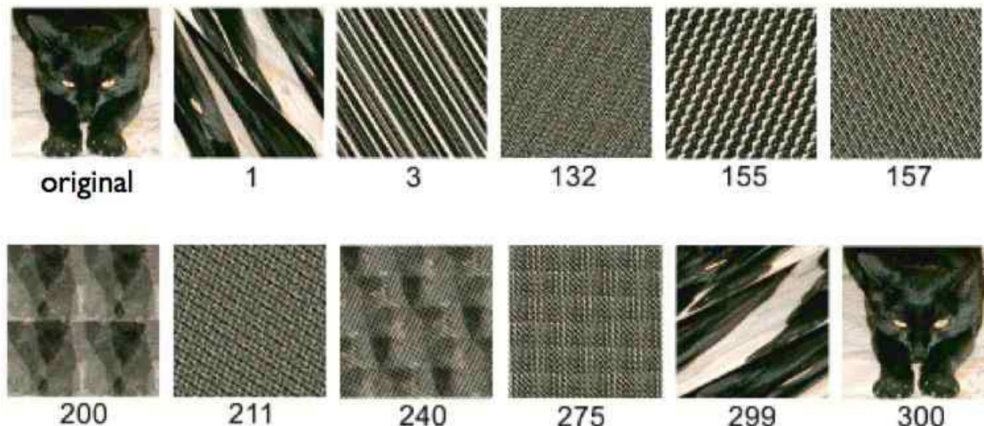
Figure 3.10: The Arnold cat map applied to an image of 150 \times 150 pixels. After 300 iterations, the image repeats itself. (Source: Wikipedia)
