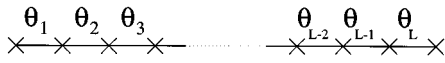
FIG. 1. Schematic representation of a 1D Josephson-junction array. The crosses represent the tunnel junctions between superconducting segments, and \theta_i are the phases of the superconducting order parameter in the latter.
