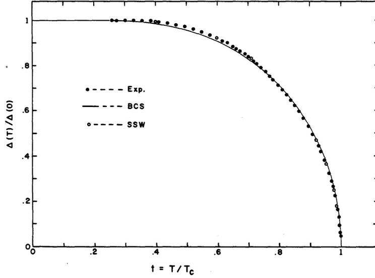
Figure 12.5: Temperature dependence of the energy gap in Pb as determined by tunneling *versus* prediction of BCS theory. From R. F. Gasparovic, B. N. Taylor, and R. E. Eck, *Sol. State Comm.* **4**, 59 (1966). Deviations from the BCS theory are accounted for by numerical calculations at strong coupling by Swihart, Scalapino, and Wada (1965).
