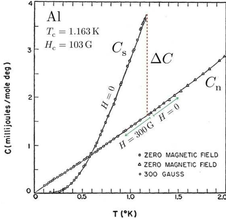
Figure 12.6: Heat capacity in aluminum at low temperatures, from N. K. Phillips, *Phys. Rev.* 114, 3 (1959). The zero field superconducting transition occurs at  $T_c = 1.163$  K. Comparison with normal state  $C$  below  $T_c$  is made possible by imposing a magnetic field  $H > H_c$ . This destroys the superconducting state, but has little effect on the metal. A jump  $\Delta C$  is observed at  $T_c$ , quantitatively in agreement BCS theory.
