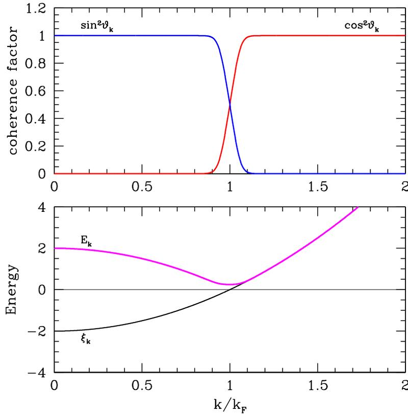
Figure 12.4: Top panel: BCS coherence factors  $\sin^2 \vartheta_k$  (blue) and  $\cos^2 \vartheta_k$  (red). Bottom panel: the functions  $\xi_k$  (black) and  $E_k$  (magenta). The minimum value of the magenta curve is the superconducting gap  $\Delta_0$ .
