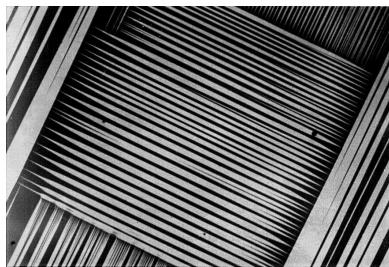
Fig. 11.11 Martensite. A particularly nice example of a martensitic structure, from Chu [30]. The light and dark stripes represent two different martensitic variants—that is, the crystal going through the phase transition can stretch in different directions, and the two colors indicate that the local lattice is stretching along two different axes. The tilted square region occupying most of the photograph could not change its overall shape without putting incompatible strains on the neighboring domains. By making this striped pattern, or laminate , the martensite can form an average of the different stretching directions that gives zero net strain.
