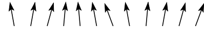
Fig. 9.9 Magnets: spin waves. Magnets break the rotational invariance of space. Because they resist twisting the magnetization locally, but do not resist a uniform twist, they have low-energy spin wave excitations.
