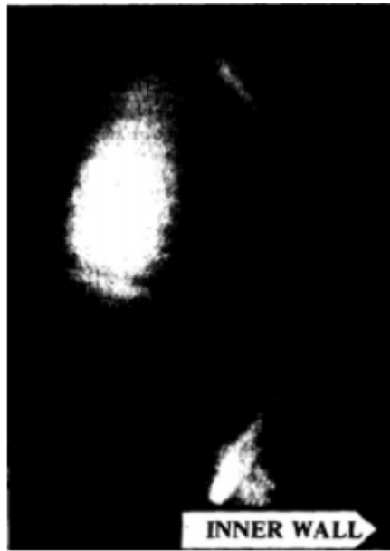
Figure 7: Illuminated coherent filamentary structures seen from the gas-puffing position in ASDEX. Taken from [1].
