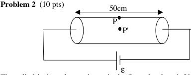
The cylindrical conductor shown in the figure has length 50cm, cross-sectional area  $1 \text{mm}^2$  and is made of Cu, with resistivity  $1.7 \times 10^{-8}$  ohm-meter. The emf  $\epsilon$ =0.2V. Assume the other wires in the circuit have zero resistance.
