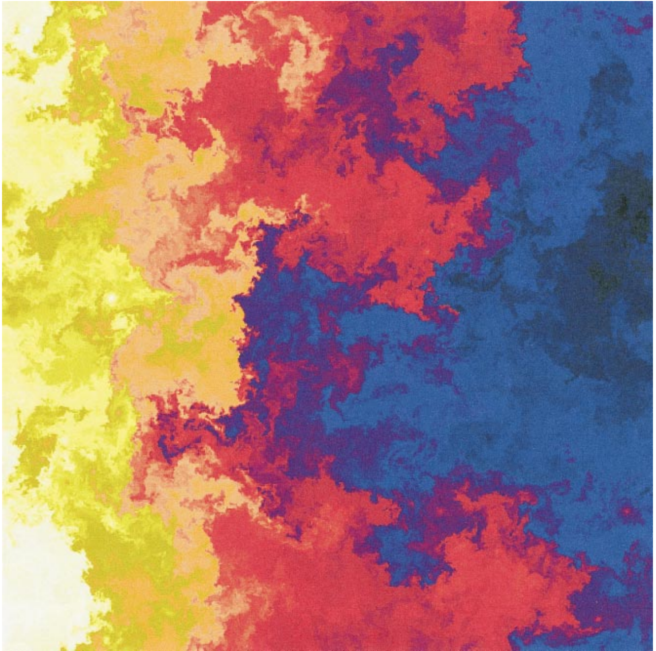
FIG. 6. A typical snapshot of a scalar field transported by a turbulent flow.
