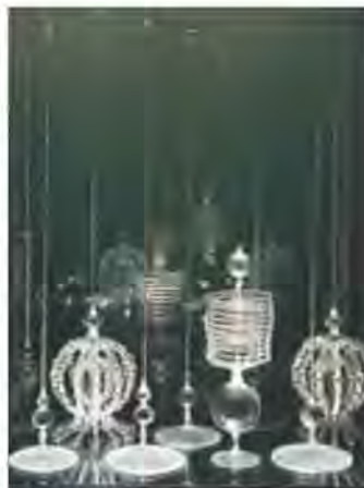
FIGURE 17-4 Thermometers built by the Accademia del Cimento (1657–1667) in Florence, Italy, are among the earliest known. These sensitive and exquisite instruments contained alcohol, sometimes colored, like many thermometers today.
