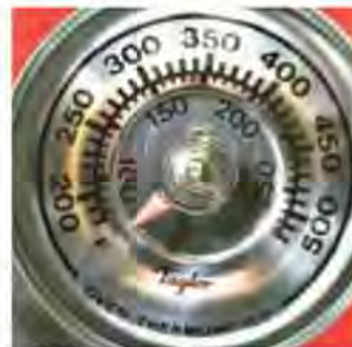
FIGURE 17-6 Photograph of a thermometer using a coiled bimetallic strip.
