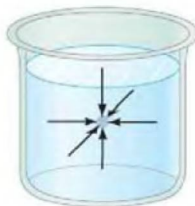
FIGURE 13-1 Pressure is the same in every direction in a nonmoving fluid at a given depth. If this weren’t true, the fluid would be in motion.
