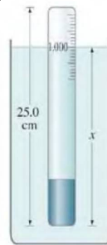
FIGURE 13–19 A hydrometer. Example 13–11.
