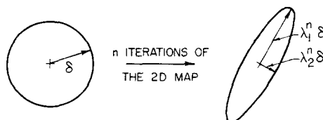
Fig. 5. n iterations of a two-dimensional map transform a sufficiently small circle of radius \delta approximately into an ellipse with major and minor radii (\lambda_1)^n \delta and (\lambda_2)^n \delta , where \lambda_1 and \lambda_2 are the Lyapunov numbers.
