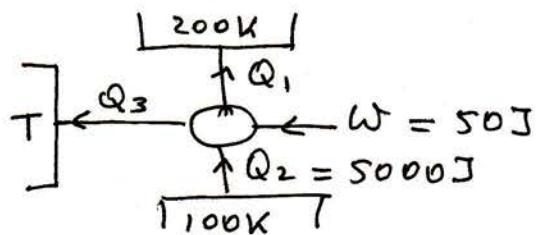
$$(a) Q_1 = 5049 \text{ J} \Rightarrow Q_3 = 1 \text{ J}, \text{ so } Q_2 + W = 5050 \text{ J} = Q_1 + Q_3$$
