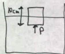
The buoyant force  $F_B$  equals the weight, since the block floats.
