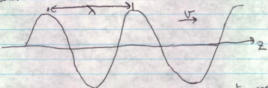
$k = \frac{2\pi}{\lambda}$     $T = \text{Period} = \text{Time taken for wave to execute 1 complete oscillation at a fixed point in } z = \frac{\lambda}{v}$
