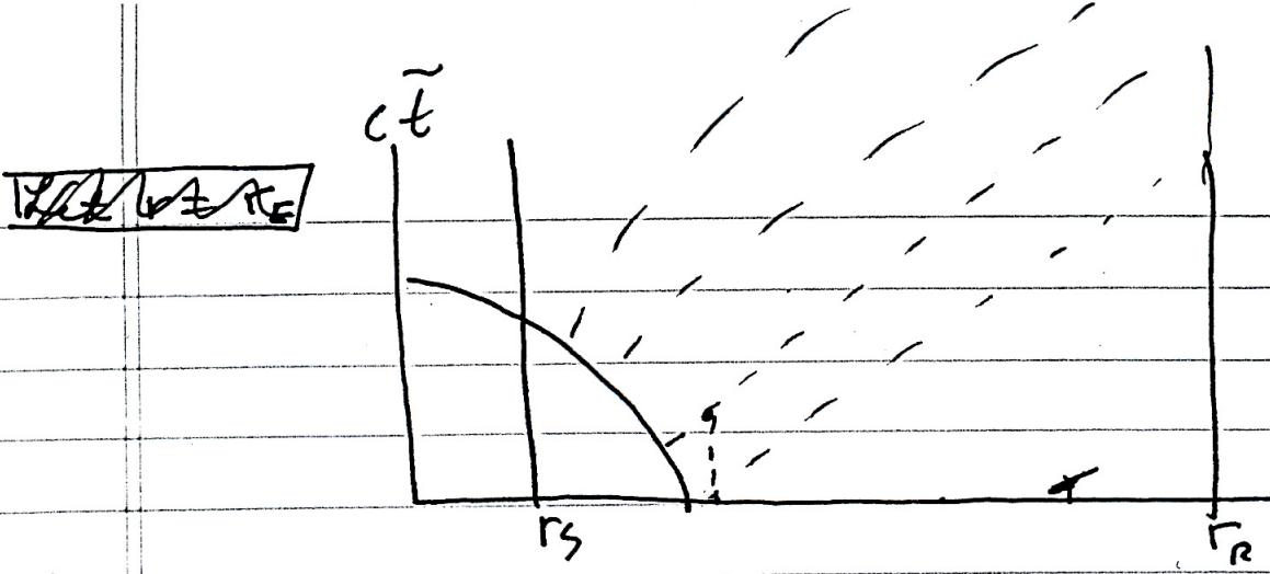
Signals detected at  $(r_R, ct_R)$  but emitted at  $(r_E, ct_E)$ .
