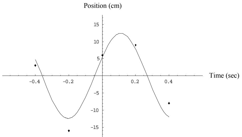
For 3 of 5 data points, the fit is pretty good with “a couple of centimeters” as the tolerance. However, the fit is not as good near the peaks.
