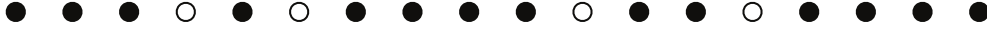
Figure 5.1: Partitioning N bosons into J possible states ( N = 14 and J = 5 shown). The N black dots represent bosons, while the J - 1 white dots represent markers separating the different single particle populations. Here n_1 = 3 , n_2 = 1 , n_3 = 4 , n_4 = 2 , and n_5 = 4 .
