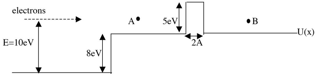
1000 electrons of kinetic energy  $10\text{ eV}$  are incident from the left and encounter the potential  $U(x)$  shown in the figure.
