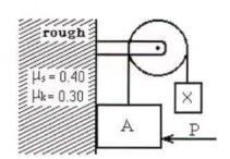
7) Block A of mass 6 kg and block X are attached to a rope which passes over a pulley, as indicated in the figure above. A 50 N force is applied horizontally to block A, keeping it in contact with a rough vertical face. The coefficients of static and kinetic friction are  $\mu_S = 0.40$  and  $\mu_K = 0.30$ . The pulley is light and frictionless. The mass of block X is set so that block A is on the verge of slipping upward. The mass of block X is closest to:
