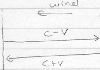
$$t_1 = \frac{d}{v} = \frac{L}{c-v} + \frac{L}{c+v} = \boxed{\frac{2L}{c} \left( \frac{1}{1-\frac{v^2}{c^2}} \right)}$$
