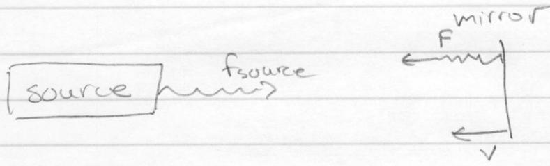
The mirror reflects light at the frequency which it observes, or  $f_{\text{ref}} = \sqrt{\frac{c+v}{c-v}} f_{\text{source}}$  and is
