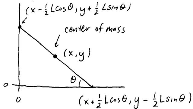
Constraints :  $G_1(x, y, \theta) = x - \frac{1}{2}L \cos \theta$  (left edge on wall)
