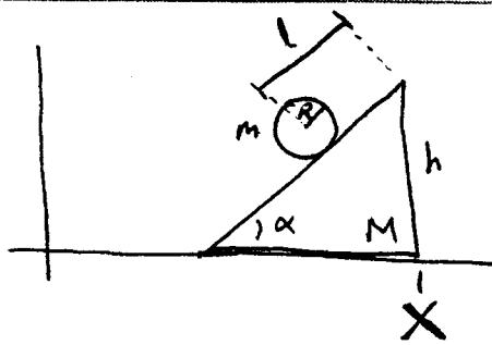
$$\begin{aligned} l &= R\phi \quad ; \quad \phi = \text{angle hoop rolls through} \\ x_{cm} &= X - l \cos \alpha \\ y_{cm} &= h + R - l \sin \alpha \\ \dot{x}_{cm} &= \dot{X} - R \cos \alpha \dot{\phi} \\ \dot{y}_{cm} &= - R \sin \alpha \dot{\phi} \end{aligned}$$
