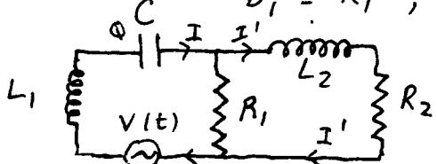
$$\begin{aligned} \frac{Q}{C} + L_1 \ddot{Q} + R_1(\dot{Q} - I') &= V(t) \\ L_2 \dot{I}' + R_2 I' + R_1(I' - \dot{Q}) &= 0 \end{aligned}$$
