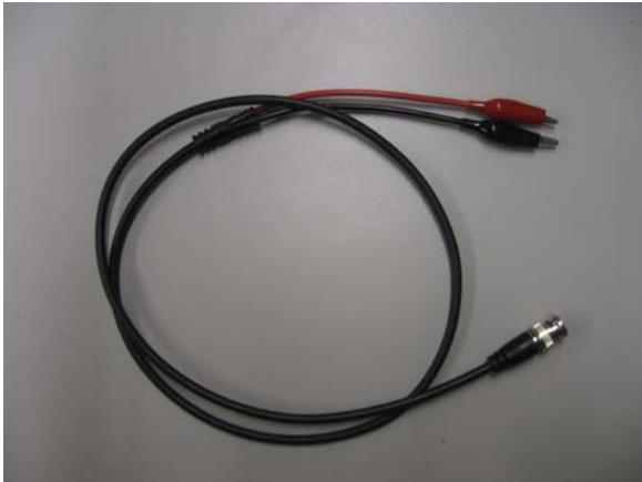
Figure 1 The top right image is the “alligator clip” end of the cable pictured above. The lower right image is the BNC cable end of the female type.
