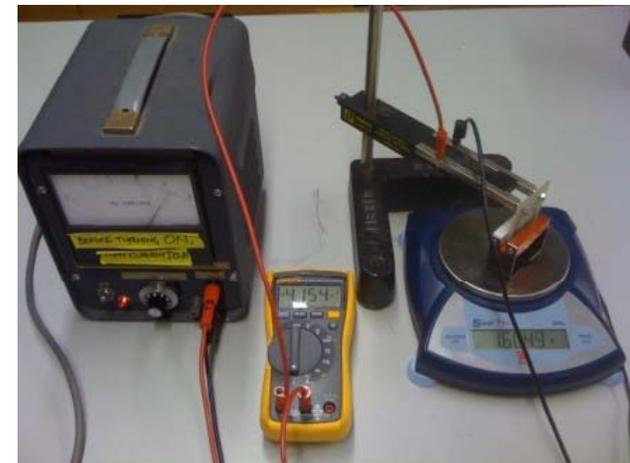
Determine the magnetic field of the magnet by measuring the force on a current in the field. Choose several hairpins of different lengths. For each hairpin choose several different currents. Measure the mass difference from the scale and calculate the Lorentz force.
