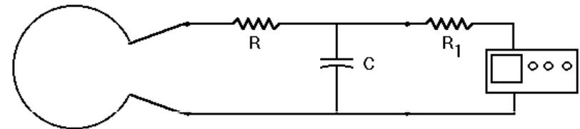
actual decay time constant is  $R_2 C$ , where  $R_2 = \frac{R_1 R}{R_1 + R}$
