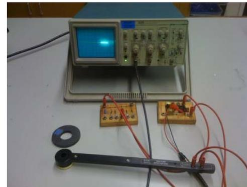
the output voltage for a flip coil moved rapidly out of a magnetic field region and integrated by an RC circuit followed by discharge of the capacitor
