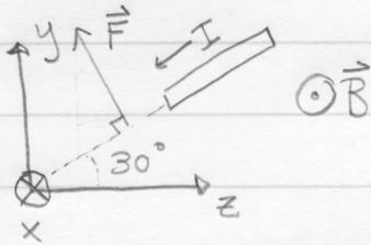
Wire in a magnetic field:  $I = 3.5\text{A}$ ,  $B = 0.5\text{T}$ ,  $l = 1.2\text{m}$
