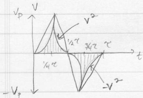
$$\begin{aligned} \int_0^T V^2 dt &= 4 \int_0^{1/4T} V^2 dt = 4 \int_0^{1/4T} (V_p^2)^2 dt \\ &= 4 \left( \frac{4V_p^2}{\pi} \right)^2 \frac{1}{3} \left( \frac{\pi}{4} \right)^3 \\ &= \frac{1}{3} V_p^2 T \end{aligned}$$
