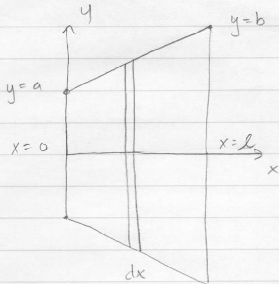
$$R = \int_{\text{cone}} dR = \int_{x=0}^{x=l} \rho dx \quad A = \pi y^2, \quad y = \left(\frac{b-a}{l}\right)x + a$$
