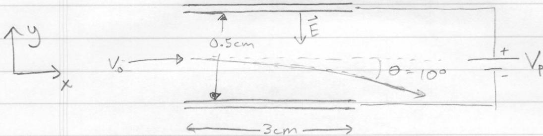
charged particle,  $\Delta V_{acc} = 15,000 \text{ V}$  accelerating voltage, deflected by charged plates, what  $V_p$  to get  $\theta = 10^\circ$ ?
