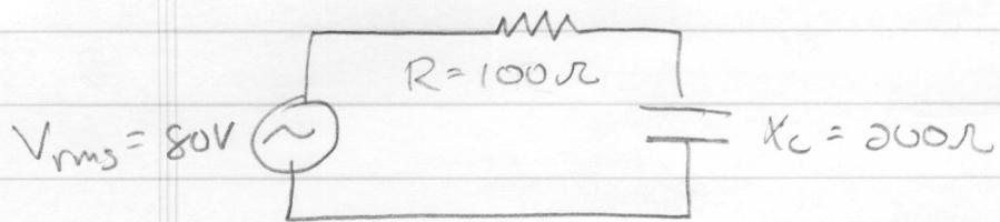
$$I_{rms} = \frac{V_{rms}}{Z}, \quad Z = \sqrt{R^2 + X_C^2}$$
