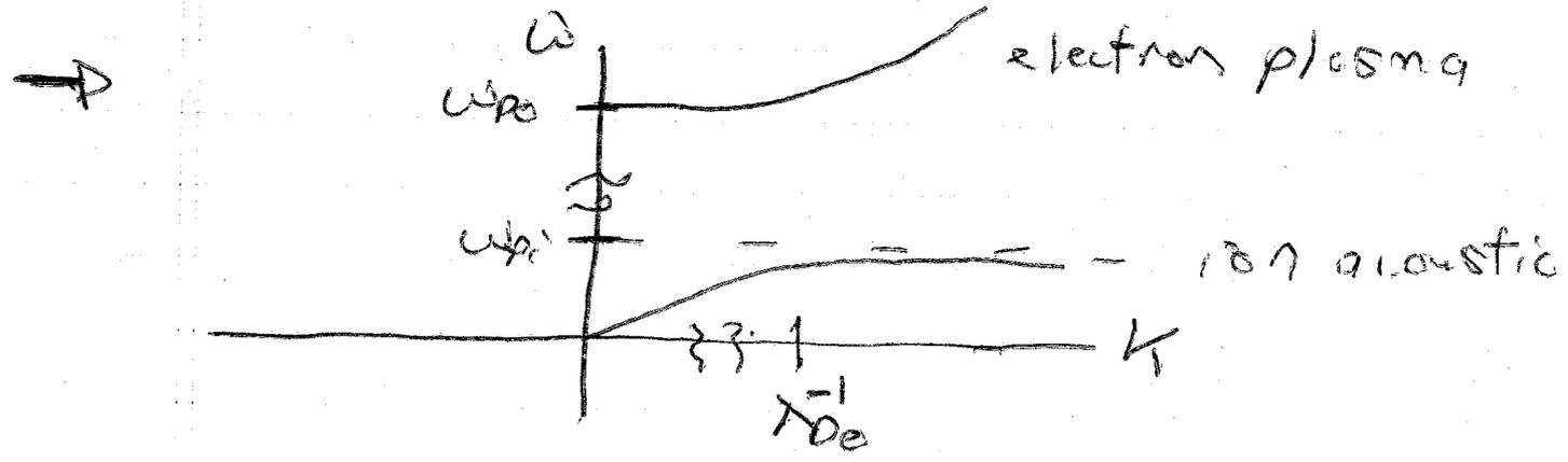
Basic modes (electrostatic) of un-magnetized plasma.
