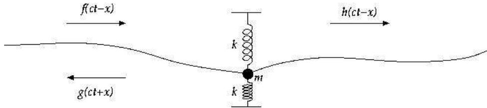
Figure 1: A string with a mass point connected to springs. An incident wave gives rise to reflected and transmitted components.
