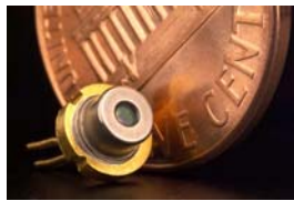
Laser diode Used in cd players etc.
