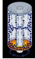
centrifugal separation gaseous \text{UF}_6
