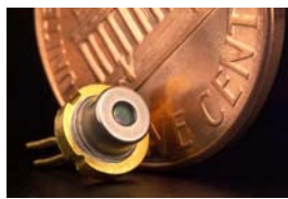
Laser diode Used in cd players etc.
