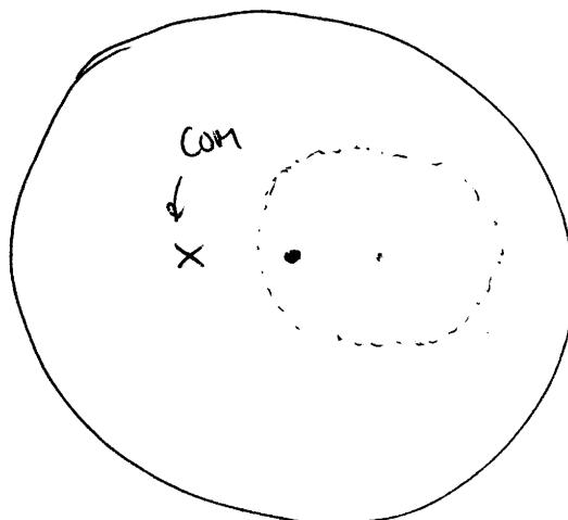
(P73) Momentum must be conserved , so when the passenger climbs downward , the balloon must move upward
