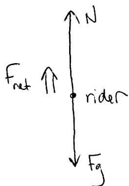
At the bottom, the normal force increases so that the net force is toward the center.
