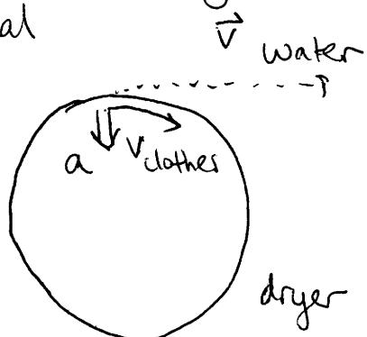
(Q10) If you are interested in the force exerted on an object in the centrifuge, you not only need to know the rotational speed, but also the distance from the center of the centrifuge. The force exerted on an object in a centrifuge is the centripetal force which depends on the mass of the object, the radius of the orbit and the rotational speed.
