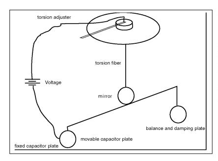
A simple and accurate method to measure the force is to attach one of the plates to a torsion pendulum, while keeping the other plate fixed. The figure shows a capacitor plate electrically connected to the left arm of the torsion pendulum. (An identical plate is attached to the right arm to balance the pendulum and to pendulum damp the oscillations by placing it in water).
